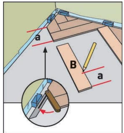
For the last plank, take a measurement (a) and mark it on your B plank.
