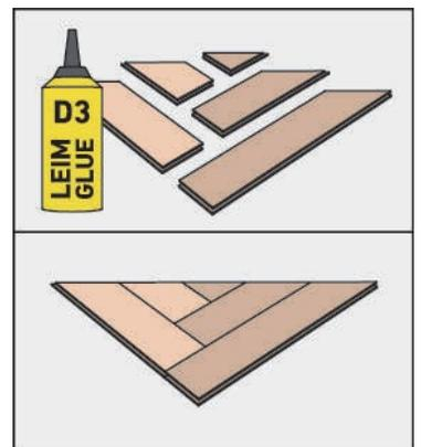
You're left with an inverted triangle. Disconnect the boards, glue, and stick back together, making your shape more sturdy.
