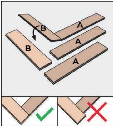
Take two B planks and three A planks. Click the first B plank into the Header Joint of the first A plank. This will form a V shape.
