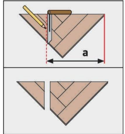
For the left-hand wall, take distance (a), mark (right-to-left) on the inverted triangle and cut. For the right-hand wall mark (left-to-right) and cut.
