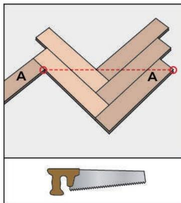
Mark a straight line from the top right corner of the third A plank to the top right corner of the fourth A plank and cut.
