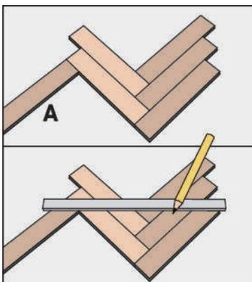
Take a fourth A plank and click the header joint in place to the second B plank.
