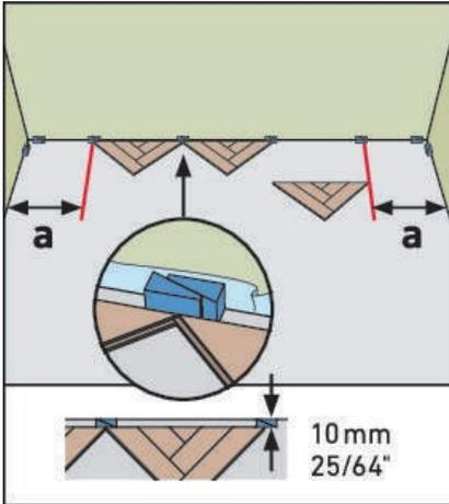
Starting from the centre of the rear wall and working outwards, place your inverted triangles. Make sure there's a 10mm gap at the back and side walls
