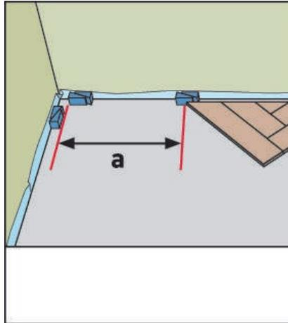
To fit the last inverted triangles against the left and right-hand wall, first measure the distance (a). Make sure your measurement stops 10mm short of the wall.
