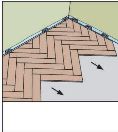
Continue working down, using B planks from right-to-left and A planks from left-to-right, applying the same methods as above.
