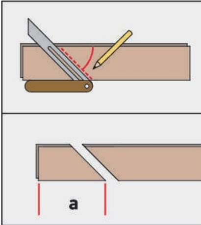
Cut measurement (a) at a 45° angle so it fits within the remaining space.
